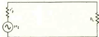
Fig. 2—Schematic diagram of the equivalent plate circuit of the output stage.
